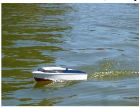
Now back to the Huntsman (Photo at left), this ran very well for a start and then got progressively slower. I put it down to battery power but when I checked the motor it was so hot it was not funny. I took it home and checked things a few days later only to find a seized motor which went on to completely fry the speed control. I now had a stuffed motor and speed
