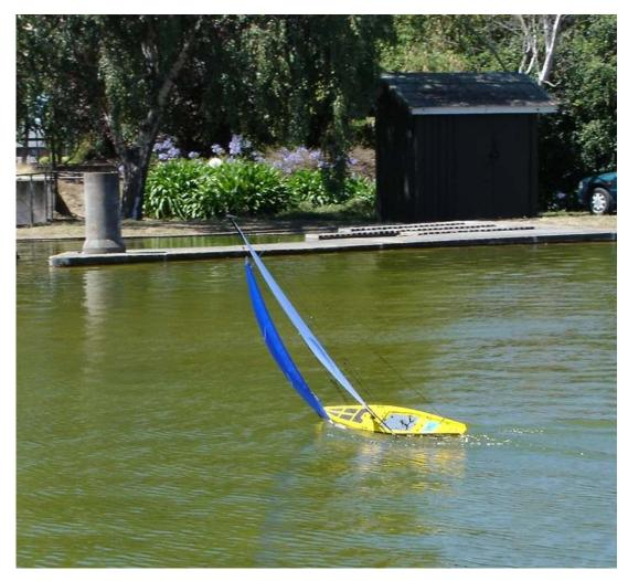
I got this yacht from HobbyKing, glass hull, all fittings and servos installed. Just needed ballast added. After a disappointing first run and a few teething problems, mainly to do with keel weight and too much rudder throw, the one meter yacht it is now running very quickly and I'm a happy chappie.
